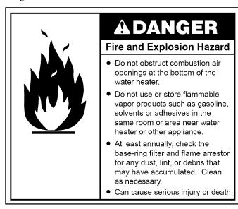
AT LEAST ANNUALLY, A VISUAL INSPECTION SHOULD BE MADE OF THE BASE-RING FILTER AND FLAME ARRESTOR. CLEAN IF LINT ACCUMULATIONS ARE NOTICED.
